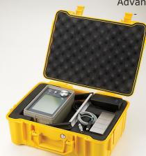
The inspection technique of alternative electromagnetic field can resolve the problem of detecting the surface cracks under thick anticorrosion layers of coating by a convenient and quick test.
